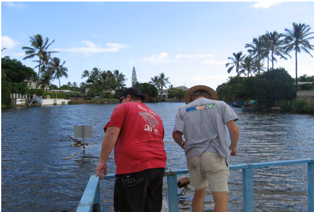
Photo 1-36 Preparation for first sediment sample at WKIP 10. Note Kaelepulu Pond entrance sign and failed turbidity curtain wrapped around it.
