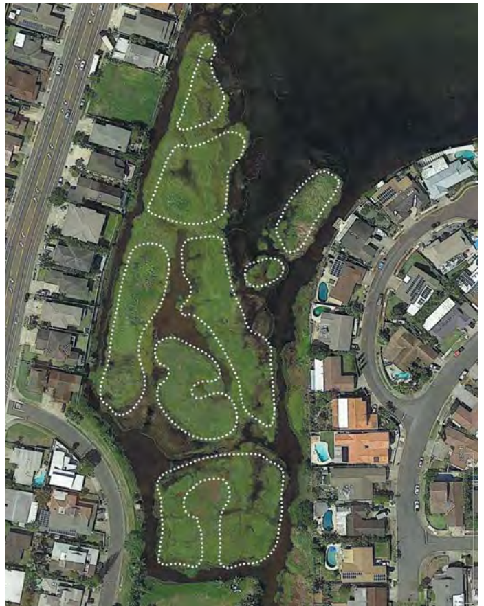
Dotted white lines indicate areas where waterways are to be opened to improve wetland habitat for fish and birds.
